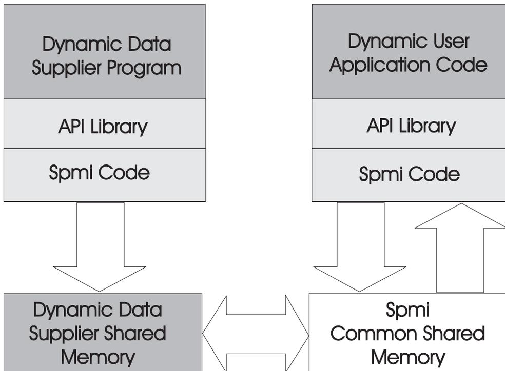
*Figure 7. Application Types. This illustration shows the DDS program on the left and the Data User Application Code on the right. Both are connected to an API library and SPMI code. The DDS program column has one way communication with the Dynamic Data Supplier Shared Memory that has two-way communication with the SPMI Common Shared Memory. The Dynamic Data Supplier Shared Memory has two-way communication with the SPMI Common Shared Memory.*
